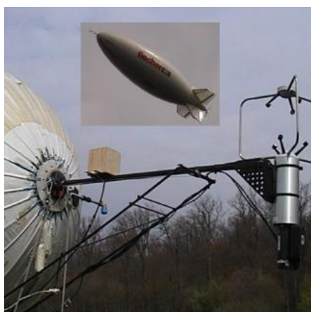
Рис. 54. MODEL 81000 SONIC ANEMOMETER ON AIRSHIP-GERMANY (Young Company)
